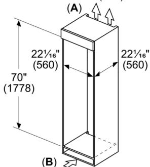
**A:** Air outlet  $\geq 31^{\prime\prime}{}^2$  ( $\geq 200 \text{ cm}^2$ )
